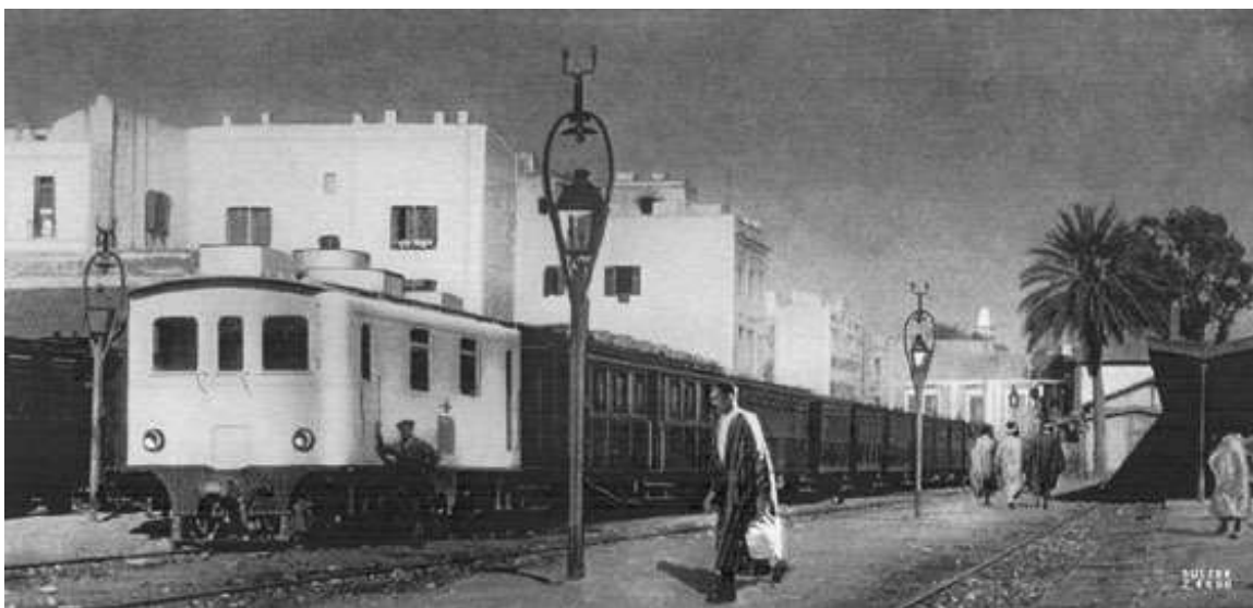
CFT Train in Tunisia in 1926 with the Sulzer diesel electric locomotive with a Sulzer four stroke 8LV21 engine of 250BHP driving a direct current dynamo of 145kW with a maximum voltage of 800V.
